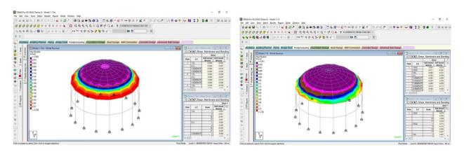
Fig 9:Maximum absolute plate stress of model no.1
