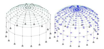
Fig 1: Monolithic dome structure geometry
