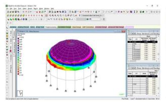
Fig 11:Maximum absolute plate stress of model no.3
